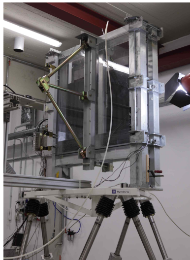
Figure 1: Experimental set-up for the sloshing-tank experiments.
