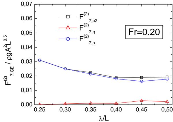
Fig. 7. 2<sup>nd</sup>-order generalized excitation for 2-node mode in vertical plane with different  $\lambda/L$  ratio.  $Fr=0.20$ .
