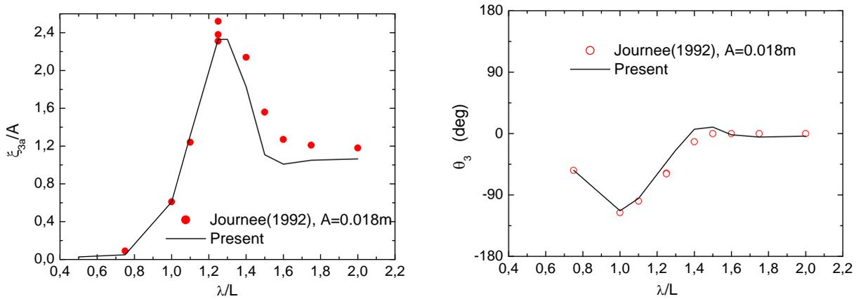
Fig.3. The amplitude and phase angle of the heave motion of Wigley hull I in head sea.  $Fr=0.3$ . The ship is restrained from surging and free to heave and pitch.
