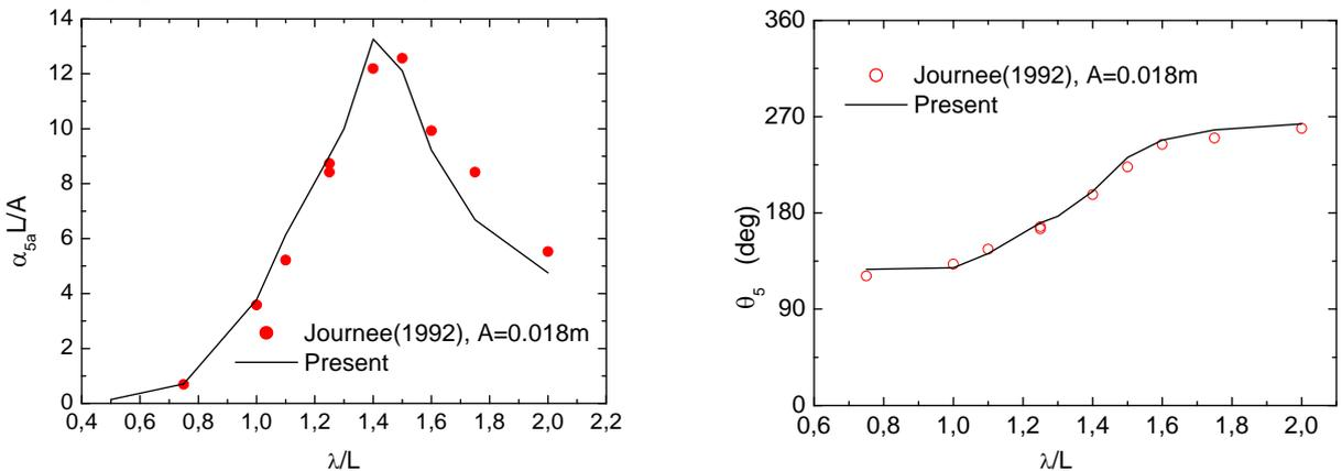
Fig.4. The amplitude and phase angle of the pitch motion of Wigley hull I in head sea.  $Fr=0.3$ . The ship is restrained from surging and free to heave and pitch.
