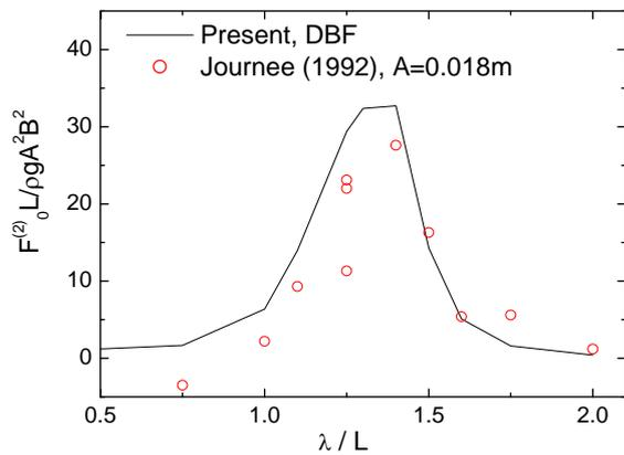
Fig. 5. Added resistance on Wigley Hull I in head sea.  $Fr=0.3$ .
