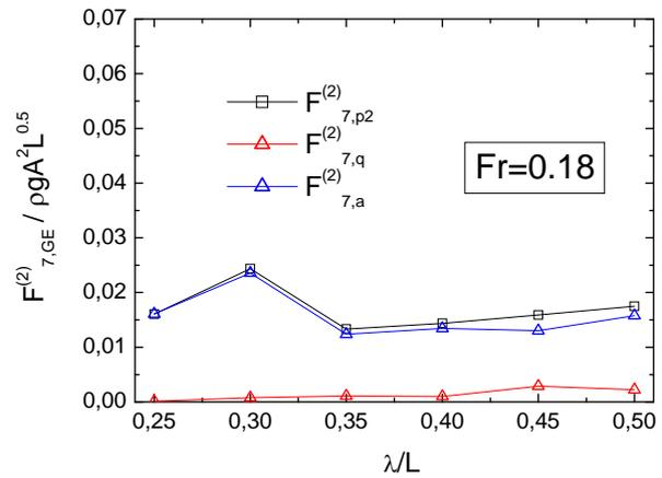
Fig. 6. 2<sup>nd</sup>-order generalized excitation for 2-node mode in vertical plane with different  $\lambda/L$  ratio.  $Fr=0.18$ .
