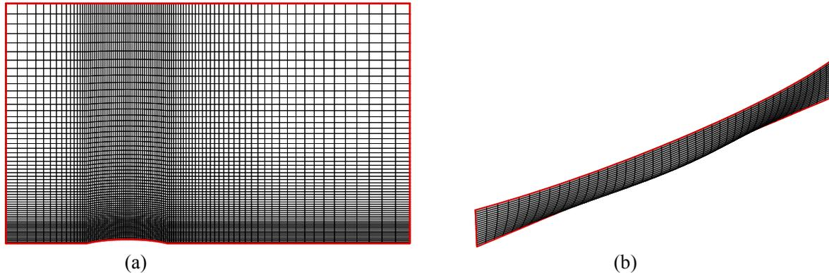
Fig.2. Meshes on the free surface and the wetted mean ship surface. Due to symmetric properties, only half of the free surface and ship surface are discretized. (a) Meshes on the half of the free surface. (b) Mesh on half of the Wigley hull.
