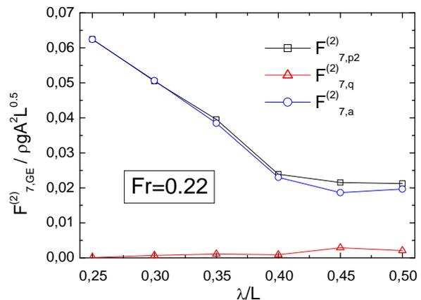
Fig. 8. 2<sup>nd</sup>-order generalized excitation for 2-node mode in vertical plane with different  $\lambda/L$  ratio.  $Fr=0.22$ .
