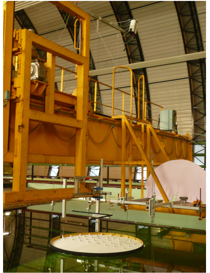
Figure 2: Camera fastened to the bridge and pointing down to the disk
