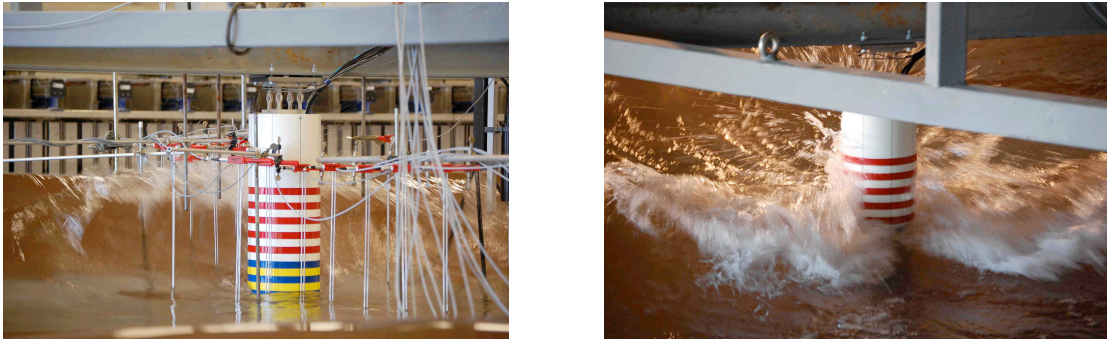
FIGURE 1. Left: Breaking wave about to hit the vertical cylinder, showing the wave gauge array and the cylinder supported from above. Right: Vertical sheet of water wrapped around the front of the cylinder during a wave impact.
