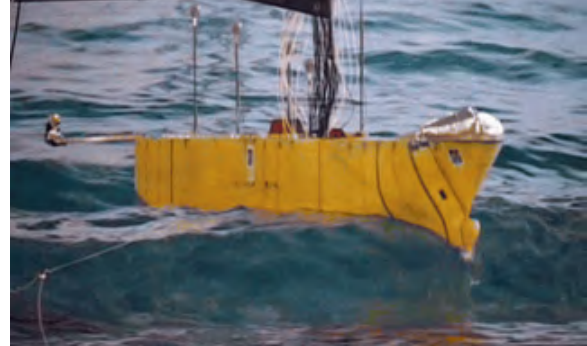
Fig. 6: View of the bulb emerging in bidirectional waves
