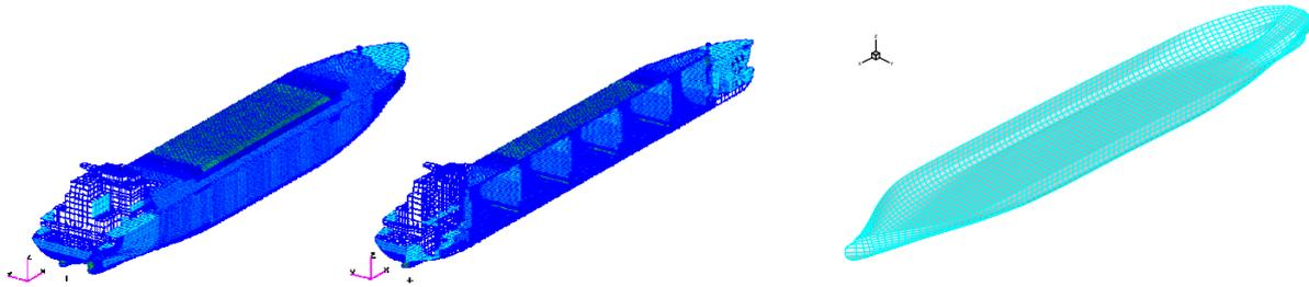
Fig.2 FEM modeling and hydrodynamic hull panels for a 330m LNG carrier
