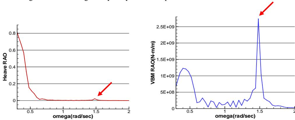
Fig.3 Heave RAO and VBM RAO at head sea: LNG carrier,  $F_n=0.18$
