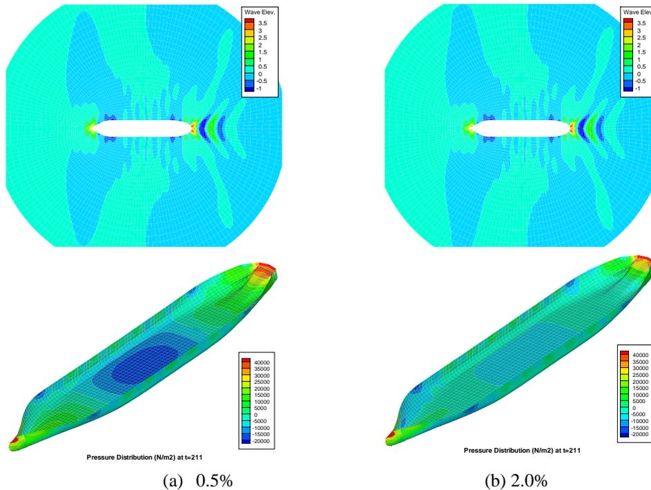
Fig.4 Effects of structural damping: LNG carrier,  $F_n=0.18$ , wave frequency at 1.48 rad/sec, instantaneous disturbed wave contour (top) and pressure contour (bottom)
