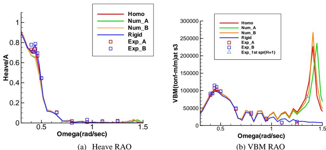
Fig.6 Heave and VBM RAOs of 10,000-TEU containership: 150deg heading, 20knots
