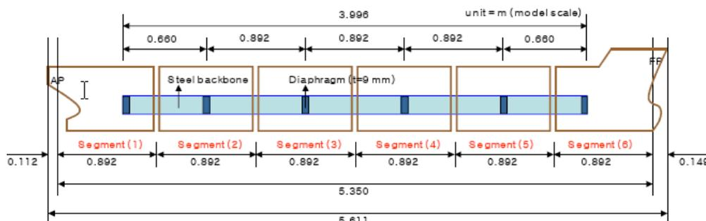
Fig.5 Segmented model for towing-tank springing test: 10,000-TEU containership, scaled for model test ([2])
