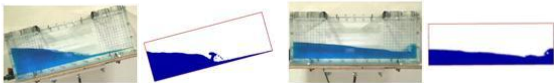
Fig.3 Comparison of water behavior between model experiment and MPS method for a rectangular tank
