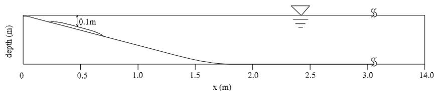
Figure 5: Scheme of landslide model in Sue (2007)
