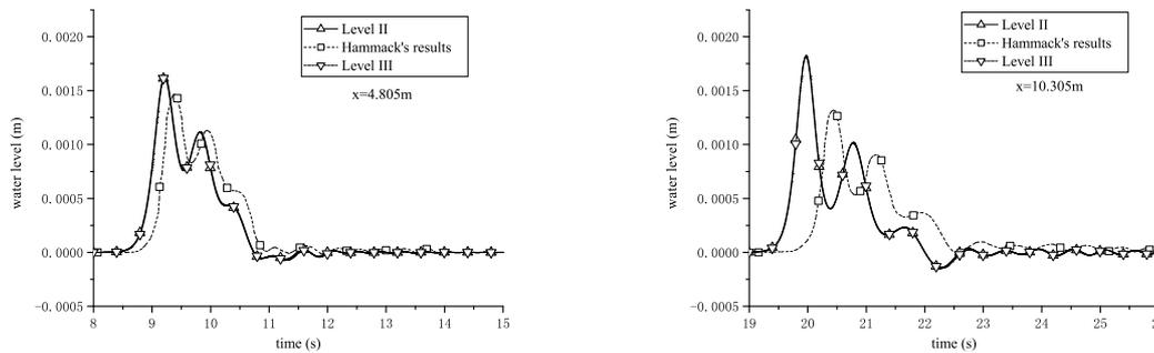
Figure 4: Free surface elevations in the downstream positions  $x = 4.805m$  (left) and  $x = 10.305m$  (right)
