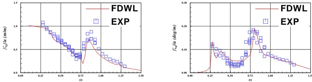
Fig. 5. Sway and yaw RAO in beam sea ( $U=0$ ) with yaw mooring moment and artificial damping
