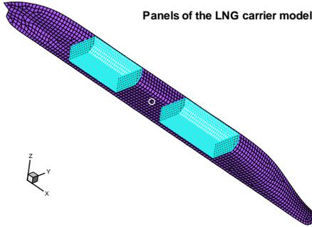
Fig. 1. Hull and tank panels of the model
