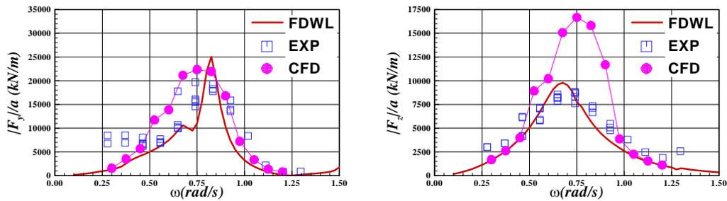
Fig. 6. Amplitude of the lateral and vertical hydrodynamic forces on the tank wall for the LNG carrier in beam sea ( $U=0$ )
