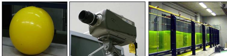
A floater (left) falls over a height  $h$  onto an initial flat free surface. A fast camera (center) records the final stage of the drop in air and the whole fluid-structure interaction up to a possible rebound. The camera works at 1000 frames per second. The water is coloured with fluorescein (right) in order to improve the diffusion of light into the liquid. Analysis of the video recording provides most of the data for the parametric study.
