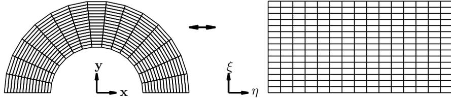
Figure 1: An example of a grid transformation.
