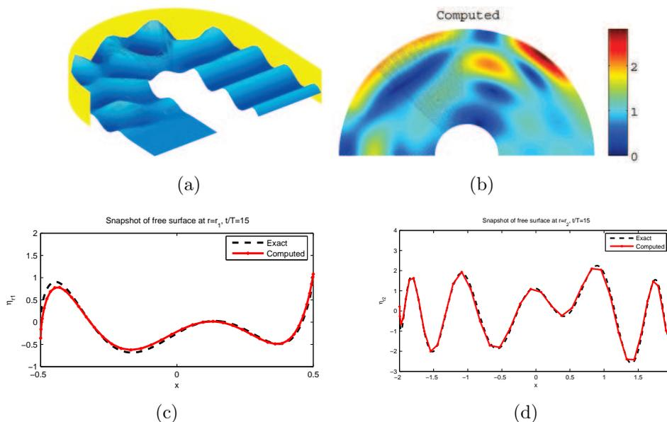
Figure 2: Propagation of waves through a semi-circular channel.
