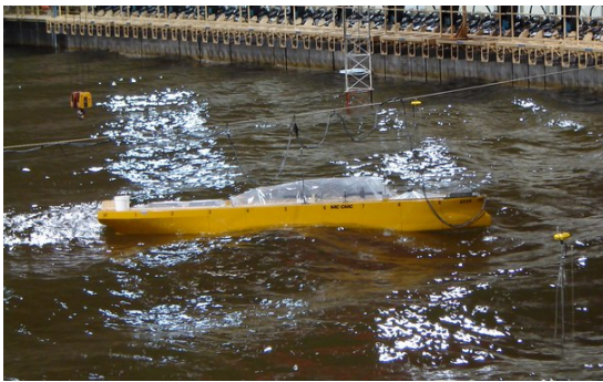
Figure 1: (up) reference plan of the basin and of the position of the model, (bottom) picture of the model in bi-directional sea-states, its bow is rotated towards positive yaw angle.
