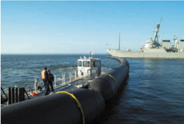
Fig 2. Dracone used as protective barrier (photo courtesy Dunlop Fabrications, Manchester, UK)
