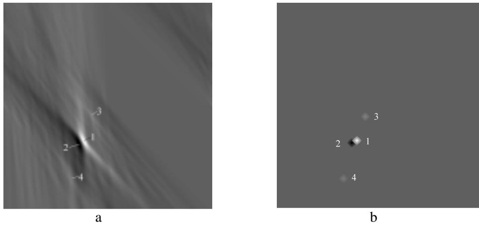
Fig. 7. Radon space of the SAR image (Fig. 1): a) raw Radon space; b) refined Radon space. Restored lines see in Fig. 2.
