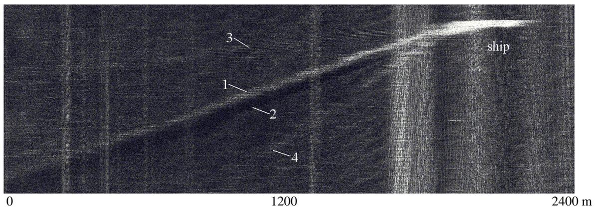
Fig. 1. Airborne ship wake image presented here was obtained by employing an X-band SAR in the course of experiments carried out in the eastern Mediterranean during light breeze. Several straight segments can be clearly identified: 1. bright wake presenting one of the two arms of the narrow V-wake; 2. long dark turbulent wake; 3-4. boundaries of the Kelvin wave-wake.
