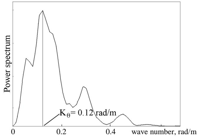
Fig. 4. Normalized power spectrum of SAR image intensity along the Kelvin cusp-line 3.
