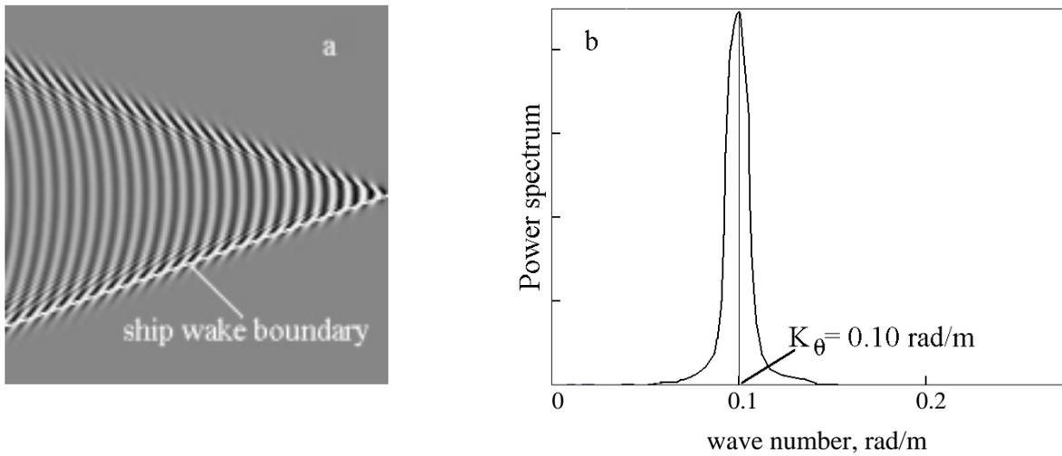
Fig. 3. Simulated longitudinal surface velocity for a ship with length  $L = 52.0$  m, beam  $B = 5.70$  m, draft  $T = 3.5$  m and speed  $U = 9.2$  m/s: a) surface velocity component; b) normalized power spectrum along the ship wake boundary.
