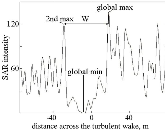
Fig. 5. SAR intensity variation in pixel brightness across the turbulent wake at some distance aft the ship (Fig.1).
