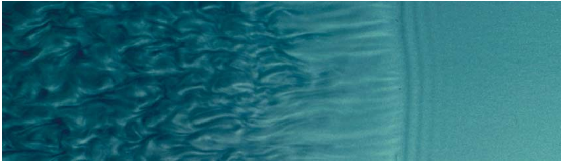
Figure 3. Flow visualisation of a “smallest breaker” in shallow water, the wave moves to the right, the water depth is approximately 7mm.
