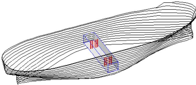
Figure 2. Modified S175 hull equipped with an ART
