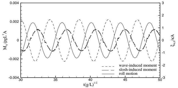
Figure 4. Time-histories of the wave-induced and slosh-induced roll moments; ART without pillars,  $\omega\sqrt{L/g} = 1.5$ ,  $A/L=0.005$
