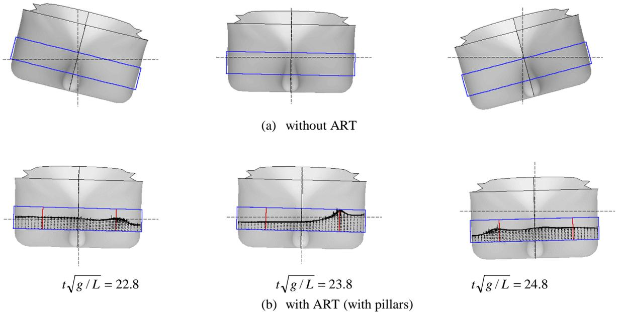
Figure 5. Instantaneous ship positions and sloshing flows at three time steps;  $\omega\sqrt{L/g} = 1.5$ ,  $A/L=0.05$ , 50% filling
