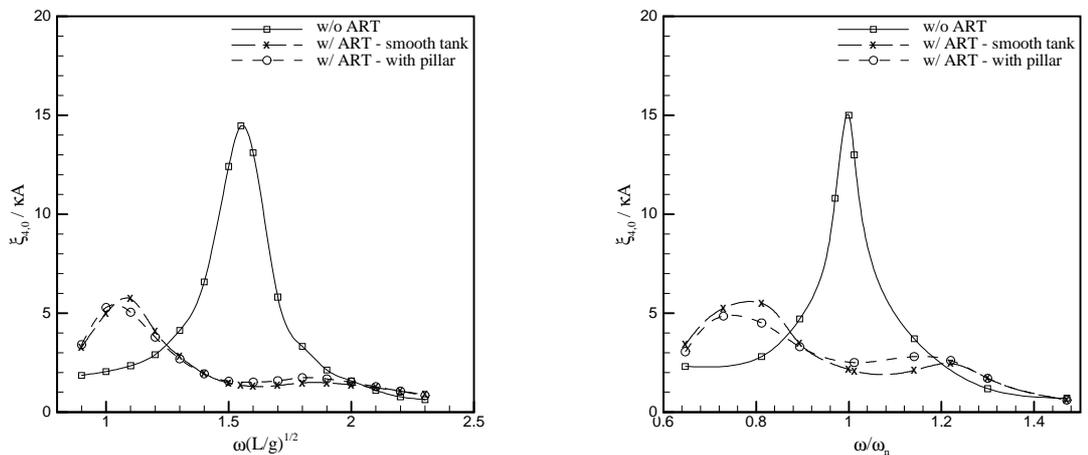
(a) Computational result for modified S175 hull
